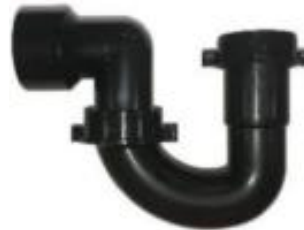
◀ 36204- 1 1/2" x 1 1/4" ABS P-Trap *1 1/4" Slip inlet x 1 1/2" Hub outlet with union joint.
