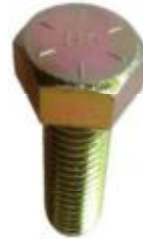
▲ 10800 - Hitch Bolt *3/4" Thread x 2" length- Grade 8 (ERB)- Use with 10801 nut.
