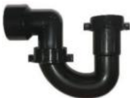
◀ 36204 -1 1/2" x 1 1/4" ABS P-Trap- *1 1/4" Slip inlet x 1 1/2" Hub outlet with union joint. Use with 38006 Tailpiece only.
